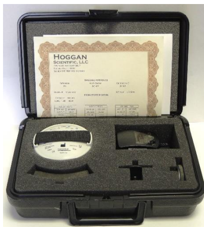
Figure 1: The microFET ® 2 device in supplied carry case
