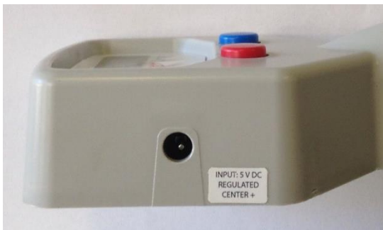
Figure 8: Device Charging Power Connector
