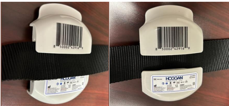
Figure 3. Strap inserted in strap guide on Test Holder
