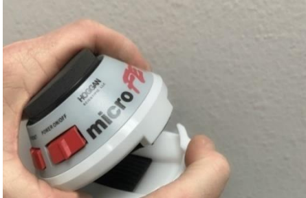
Figure 4. Attach Test Holder to Device
