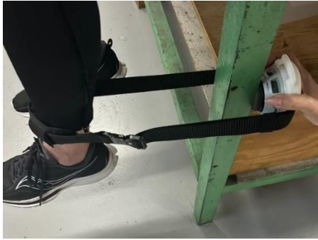
Figure 8. Muscle Test setup with device placed on fixed object.
