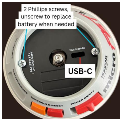
Figure 21. Device Charging and Battery Access
