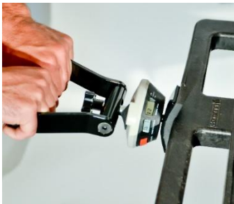
Figure 18. Example Push Test
