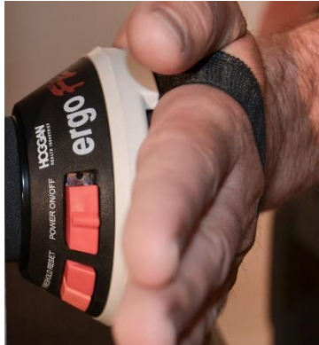
Figure 8. Compression/Push Test Device Secured to Hand
