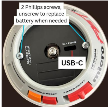
Figure 14. Device Charging and Battery Access
